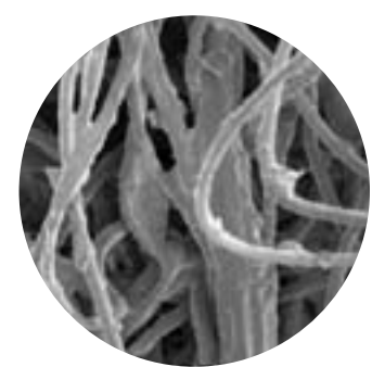
Scanning electron microscope images show the fibers of a clean cleansing cloth (top), and a cloth after cleansing (bottom), whereby the fibers have trapped and retained makeup and dirt from the skin. 5
